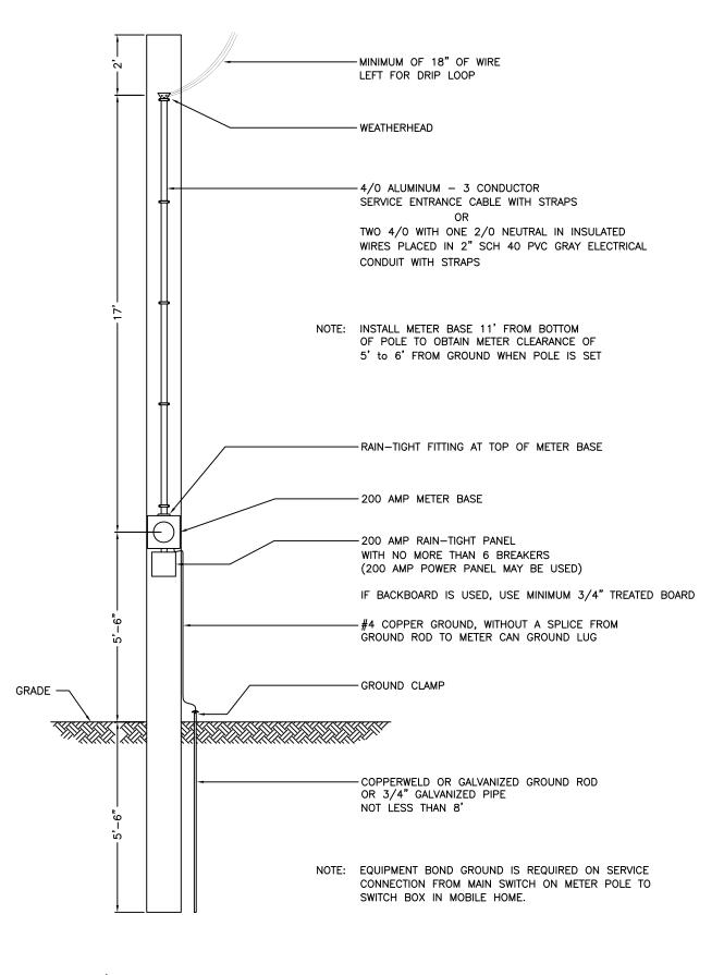
MINIMUM-30' CLASS 6 TREATED POLE LESS THAN 5 YEARS OLD AND IN SOUND CONDITION
