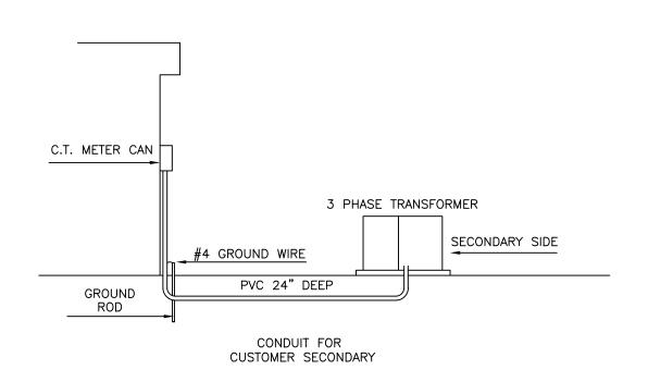
ELECTRICIAN IS REQUIRED TO PULL SEPARATE CABLES TO C.T. CABINET FROM EMC TRANSFORMER AND CUSTOMER'S SWITCH GEAR AND SPLICE THEM IN THE C.T. CABINET USING POLARIS OR COMPARABLE MULTI-TAP CONNECTOR. (MULTI-TAP CONNECTORS MUST BE PROVIDED BY ELECTRICIAN.)
